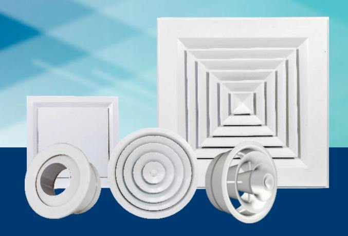
The diffusers are constructed with a heavy duty aluminium sheet and extruded profile, and powder coated for the corrosion resistance and for good aesthetical appearance. The diffusers are designed for ceiling mounting applications with effective air distribution arrangement.
