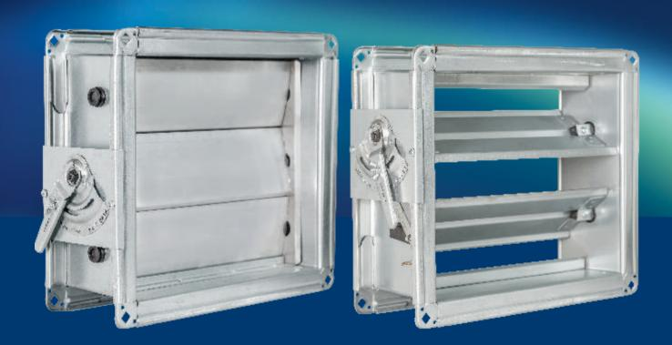
Damper are widely used in heating ventilation and air-conditioning (HVAC) application in order to maintain or control the air volume inside the duct. These dampers facilitate the air flow to each zone and each outlet to be controlled / adjusted. The damper casing is constructed with galvanized steel sheet. Damper blade which is fixed to the operating shaft can be rotated in vertical plane from full open to full close
